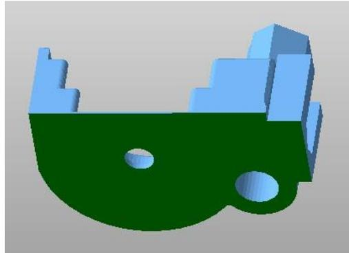
As you have seen above, the bottom was one of the areas that was too thin. It only had 0.26 mm. Rotate the view and **select the bottom**. Then go into the **Extrude** mode.
