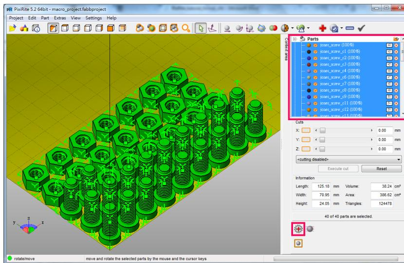
Select all the other parts (in the project tree, click on the top part, scroll down, hold Shift and click on the down part) and choose the **Automatic Part Repair** on the tabsheet.
