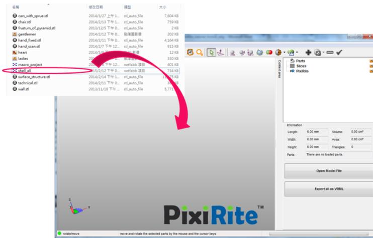
Open part of *shell\_all.fabbproject*, open the folder where you have saved the tutorial file, select the part and pull it into the PixiRite windows (The usual way via the Open/Add parts icon is possible too, of course) Make the **platform** visible: go to **View > Show platform** ◦
