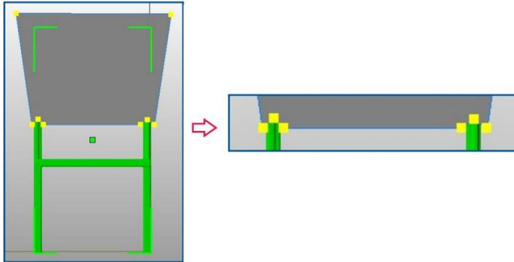
Set cutting anchors similar to the screenshot: Draw a frame around the upper third of the chair. On the bottom line of this chair, add two more anchors on each side so that two small bumps are cut out of the cutting area. When you print this chair then, these bumps will help you fit the parts perfectly together again. The notches on the bottom will make the two parts fit back together perfectly after printing. Then press **cut** to apply.
