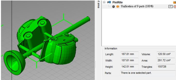
The originally 9 parts are now merged to one. This new part was automatically given a new name : *Unification of 9 parts* (see project tree) °
