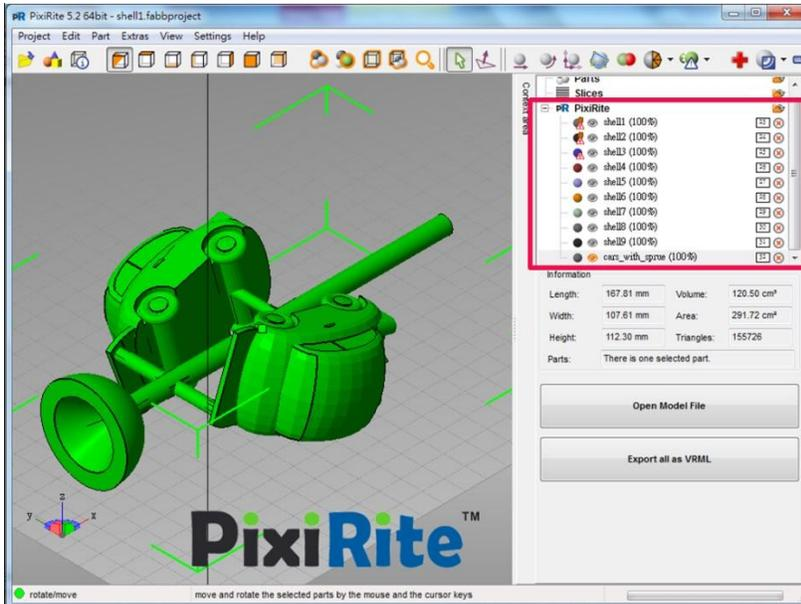
On the top right, the **project tree** lists all the parts, Click on the little
