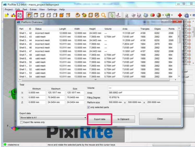
Open or continue working with the *macro\_project.fabbproject* (it's not necessary to complete Tutorial 2 before). Click on **overview** (in the toolbar) to open the dialog with all relevant details of the parts.
