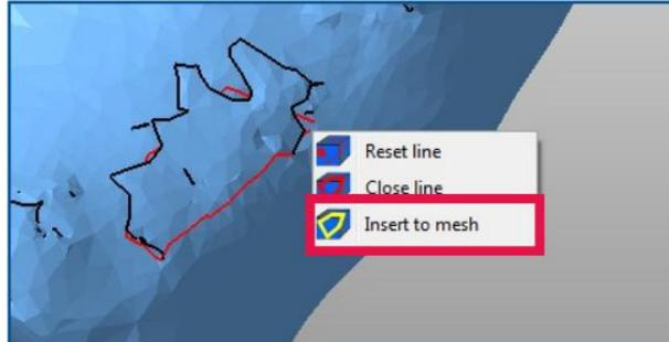
Select **Cut surfaces** and draw a line around a bump with a few mouse clicks. Try to cut out a surface as little as possible. Then right-click next to the cutting line and choose **Insert to mesh**. This way, the cut out area becomes a new shell.
