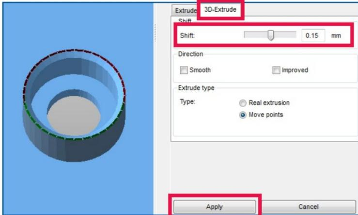
This area has a wall thickness of 0.36 mm. To extrude round surfaces, you have to switch to the **3D-Extrude** tab. Then type in *0.15 mm* (a little more than needed to be safe) in the **Shift** field and click **Apply**. Then choose **Apply repair** and **remove old part**.
