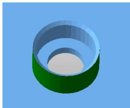
Now select the round surface in the middle of the part. Choose **Select Surfaces** again, **click on a triangle** of the surface, **rotate the view** (right mouse button), press **Ctrl** and **click on one of the other triangles** on this surface. Do that **until the whole surface is selected**. After that, go to the **extrusion mode** again.
