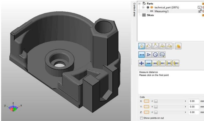
Load the part *technical.stl* and open the **measurement mode** (in the toolbar, All new measurements will be listed in the project tree.
