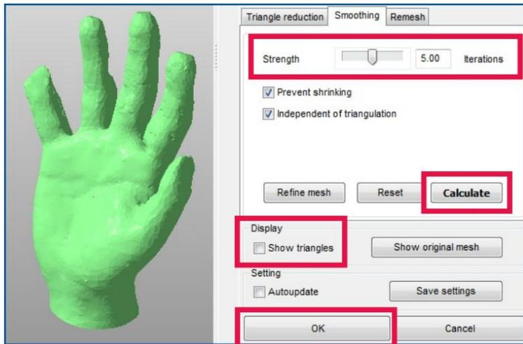
In order to have a better view of the part, **uncheck the Show triangles box**. Then set the **Strength** bar to 5.00 iterations (the more iterations, the stronger the smoothing) and press **calculate**. You now get a preview of the smoothed mesh. With pressing **Show original mesh** you can compare the original and the new mesh. Apply the smoothing with **OK** on the bottom of the tab and **Remove the old part**.
