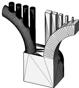
STL for example has proved itself as a very reliable file format and is now a standard in manufacturing. It does not consist of formulas but of triangles that are connected to a mesh. (Other triangle mesh formats for AM are e.g. OBJ, PLY or AMF.)
