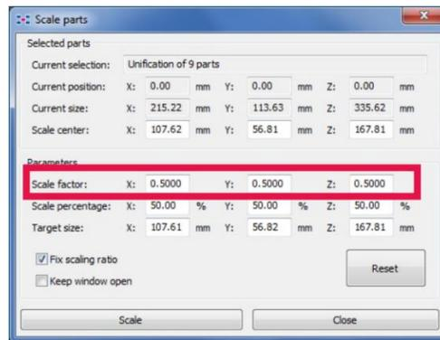
The part is relatively large. To make
