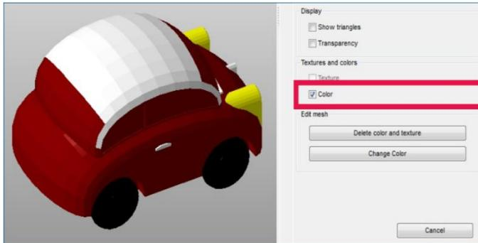
In this project the cars were originally designed with colors. Usually, STLs can't save and display color details, but this comparatively new format, called colorSTL, Display the color with the **Mesh viewer** (in the **Extras** menu). After viewing, you can **cancel** this module.
