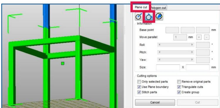
The upper part of the chair is cut off. Open the **cutting module** again, but this time, go into the **Plane cut** tab and choose the option **Create cutting plane tangential to surface**. Shift the view so you can see the chair from below.
