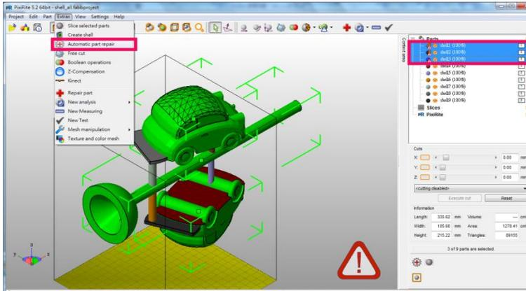
Select the broken parts *shell1* by clicking on it the project tree. Hold *Ctrl* and click on *shell2* and *shell3* to Selected 3D models are marked green in the viewing screen.
