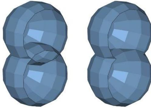
**Self-intersections:** The surface of a solid body should not contain any self-intersections. These occur whenever triangles or surfaces of one part cut through each other.
