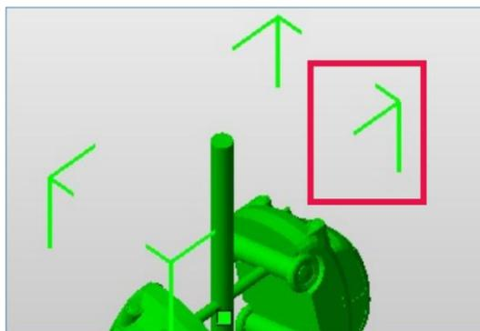
Alternatively, a part can also be rotated by holding and dragging the green corner brackets of the selected part or by entering exact values in the **rotate** dialog (in toolbar)
