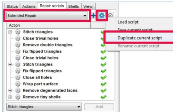
Choose the **Extended repair** and click on the little **gear** next to it in order to **duplicate** it. That way, we use the predefined powerful repair and simply add the action that we need. Name the new script *Repair and name* and press **OK**.
