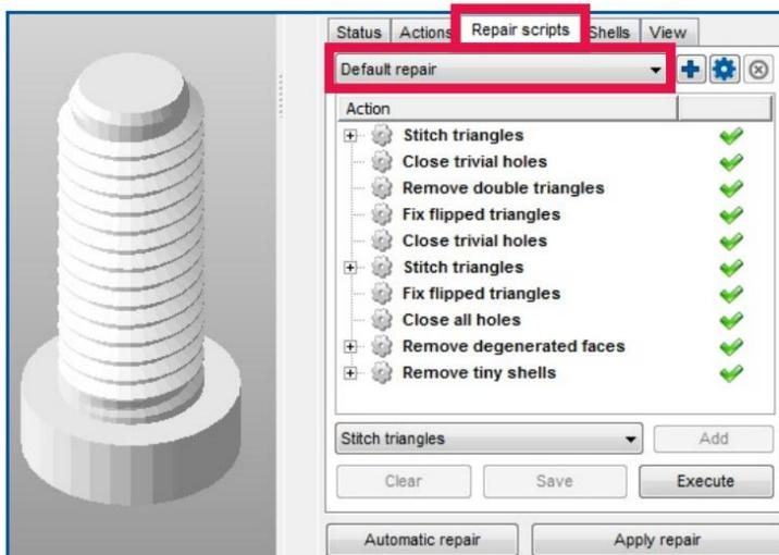
You're now in the repair mode. The toolbar on the top and the tabsheet on the right have changed – we'll go through that module later in the repair tutorials. For now, go to the **Repair scripts tab** in order to create your own macro (here called script). Expand the first dropdown menu. There are three predefined scripts: Default, Simple and Extended Repair. They're all capable of repairing a part depending on its complexity. The Extended Repair is the most powerful one.
