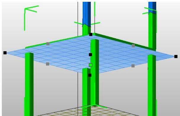
Click somewhere on the bottom of the seat and a blue cutting plane appears parallel to the bottom surface, Scale and rotate the plane until it looks similar to the screenshot:
