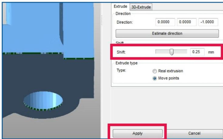
We measured 0.26 mm for the bottom wall thickness, so to make it 0.5 mm in the end, type in *0.25 mm* (a little more than needed to be safe) in the **Shift** field on the right. Then **Apply**. The bottom is now thickened.
