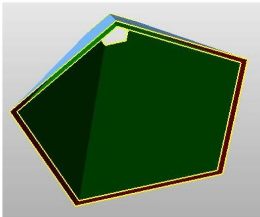
First, rotate the part so you can look at it from below. Then select the inner shell: Click on
