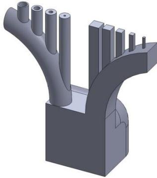
The surfaces of CAD files is determined by mathematical formulas. This works very well for constructing parts, but machines for additive manufacturing (AM) can't handle these formulas. That's why they have to be converted into another format.
