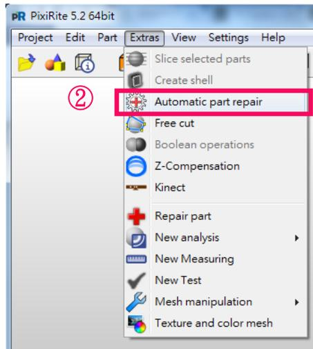
For Automatic repair the part, go into **Extras menu** and select **Automatic part repair**
