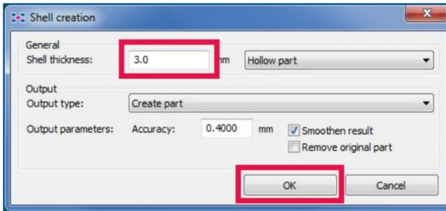
We want to create a wall thickness of 3.0mm. Enter that in the **Shell thickness** field in the Shell creation dialog and apply with **OK**.
