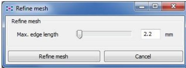
In the new dialog, pull down the maximum edge length to 2.2mm. All edges from all triangles won't be longer than 2.2mm then. The smaller the edges, the stronger the smoothing. Apply with **Refine mesh**.
