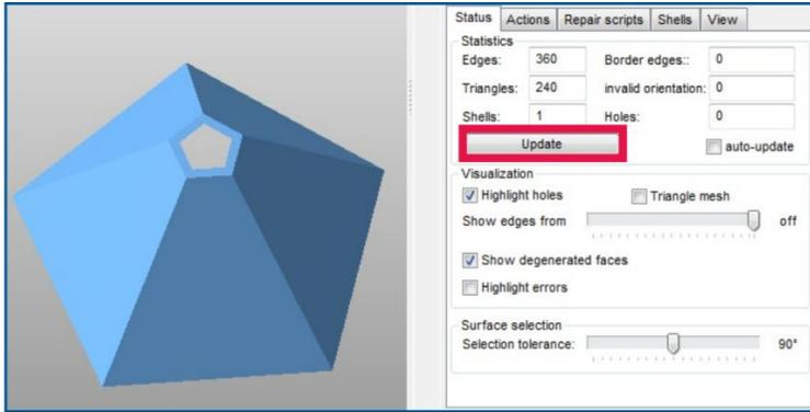
After the repair, click on **Update** again to see that there are no errors left. You have successfully repaired the part. Now press **Apply repair** and then **Remove old part**.
