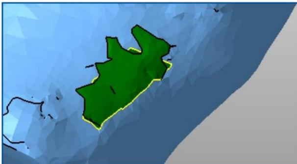
Choose the **Select Shells** mode (in the toolbar) and click on the new shell. Delete it with the **DEL** key. There's now a hole in the surface.
