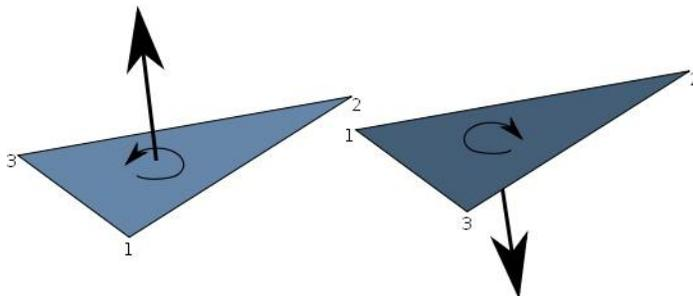
**Invalid Orientations (invalid normals):** For the conversion of triangle meshes into slice data ready for 3D printing, it is vital that the parts are oriented correctly. The orientation defines the outside and the inside of a part. In PixiRite, the inward orientation is always colored red.
