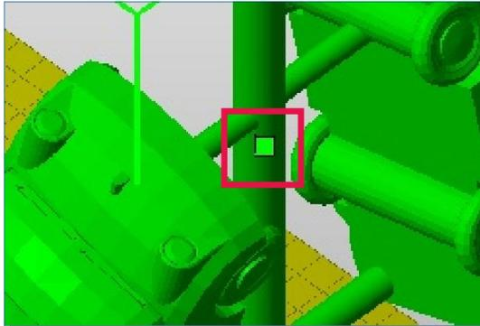
Move the part to the origin of the platform. You can do this by holding the green little square in the middle of the selected part and moving the mouse. Or to be more exact, open the
