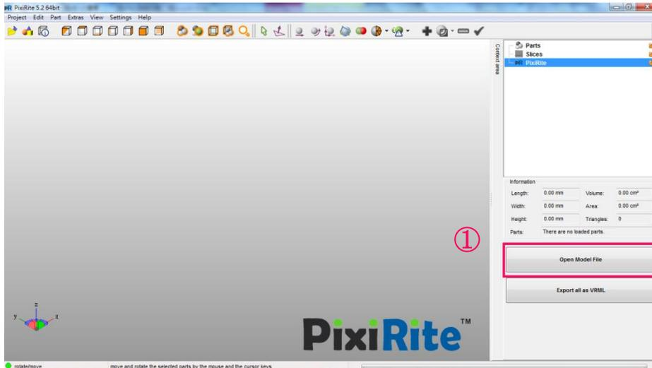
Open PixiRite and click **Open Model File** on the bottom of right column to open parts.
