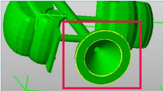
The part is now lying horizontally in the platform. To make it stand on its socket, choose the **Align to bottom plane** icon in the toolbar and **double-click on the socket's surface**. It will then stand upright.
