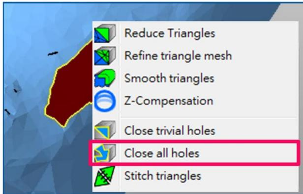
**Right-click close to the hole (= very close to the yellow line)** to open the context menu. Then choose **Close all hole**. The new triangles make a relatively flat surface. We'll later improve that. But first, **cut out all the edgy parts** as marked in the screenshot on the page before.
