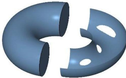
**Holes:** Parts can only be used for 3D printing, if their surface is closed (=watertight). This means they may not have any holes or open border edges.
