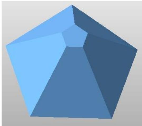
**NOTE:** After every manual repair step, you can try the automatic repair - in order to check if the rest can be done by the software. But an automatic repair still doesn't make sense for this part, Just to show you what's going wrong: here's the screenshot of it. All holes have been closed completely - though we only want to close the gap between the two shells. To undo a repair step, just press **Ctrl + Z**.
