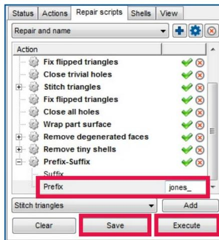
Click in the empty space behind the Prefix section and type in *Jones\_* into the new field. Apply with enter.
