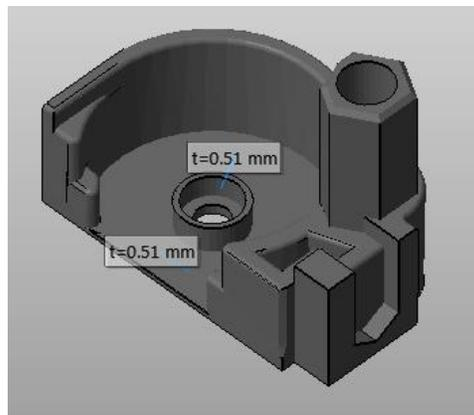
You can check if the wall thicknesses are ok now if you go to the measuring mode again. All values are at least 0.50 mm now. The part will also pass the wall thickness analysis successfully. After this, you can save or discard the result, as we'll continue with another part.
