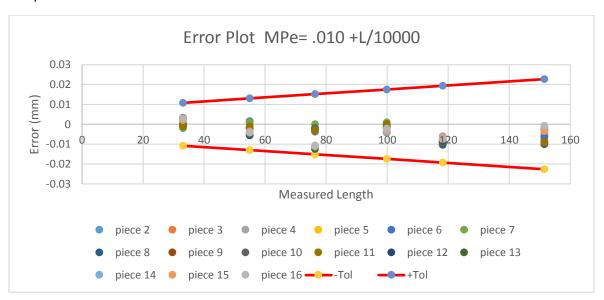
The 2 red lines represent the MPE<sub>E</sub> Tolerance. Each point is a single measurement, and the vertically stacked points represent measurements of the same ball to ball distance. For this chart we have set the tolerance, MPE<sub>E</sub>= 0.10 + L/10000. So at 0 length, we should see a maximum error of 10 microns. there are 35 ball to ball distances times 5 repetitions per machine times 3 machines represented on the chart.
