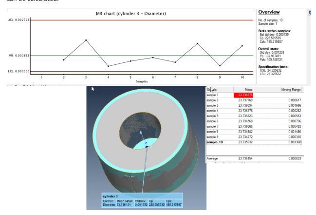
Note: Repeatability is the allowable 3 Sigma error of the measured diameter of a ring gage, repeated 10 times. Measurements are made utilizing CyberGage360's standard operating procedure, and thus include all potential hardware and software error sources.
