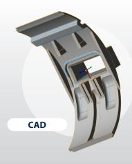
Scan generates high density point cloud data to compare to CAD models or 'golden examples.'
